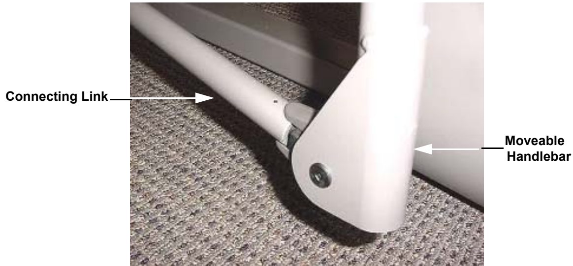
Diagram 7.16 - Moveable Handlebar, Lower End
