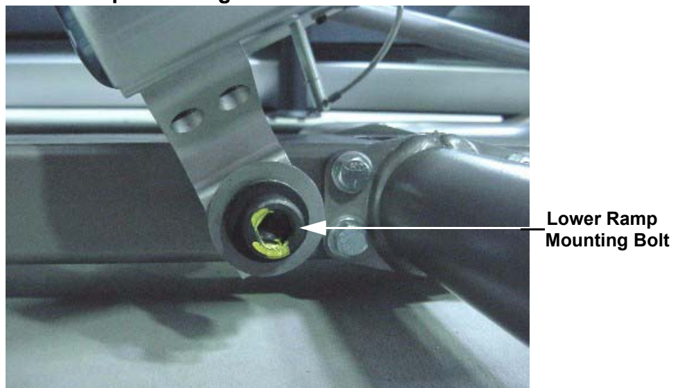
Diagram 7.14 - Lower Ramp Mounting
